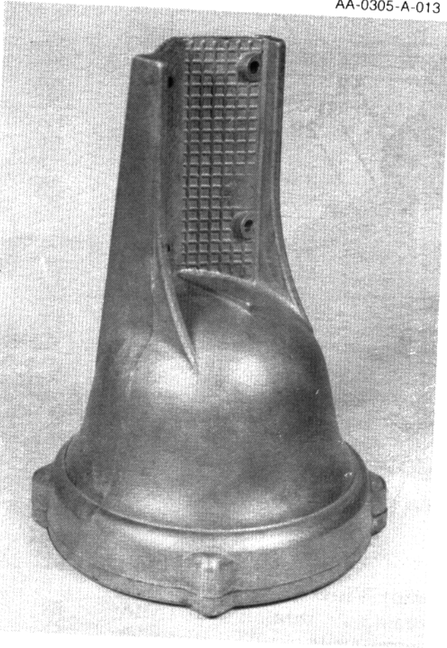
27 — Upper Mast Support — 50304-10
